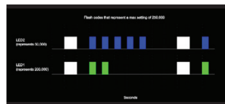
Figure 1 To change the maximum gallons setting, press and hold the button for 1 second. LED1 should turn solid green, LED2 should turn off and LED3 should flash green the number of times that corresponds to the current setting. Pressing the button for less than 1 second would increment the value, rolling over from 9 to 0. Below, Figure 2, is an example of the LEDs in this mode.
